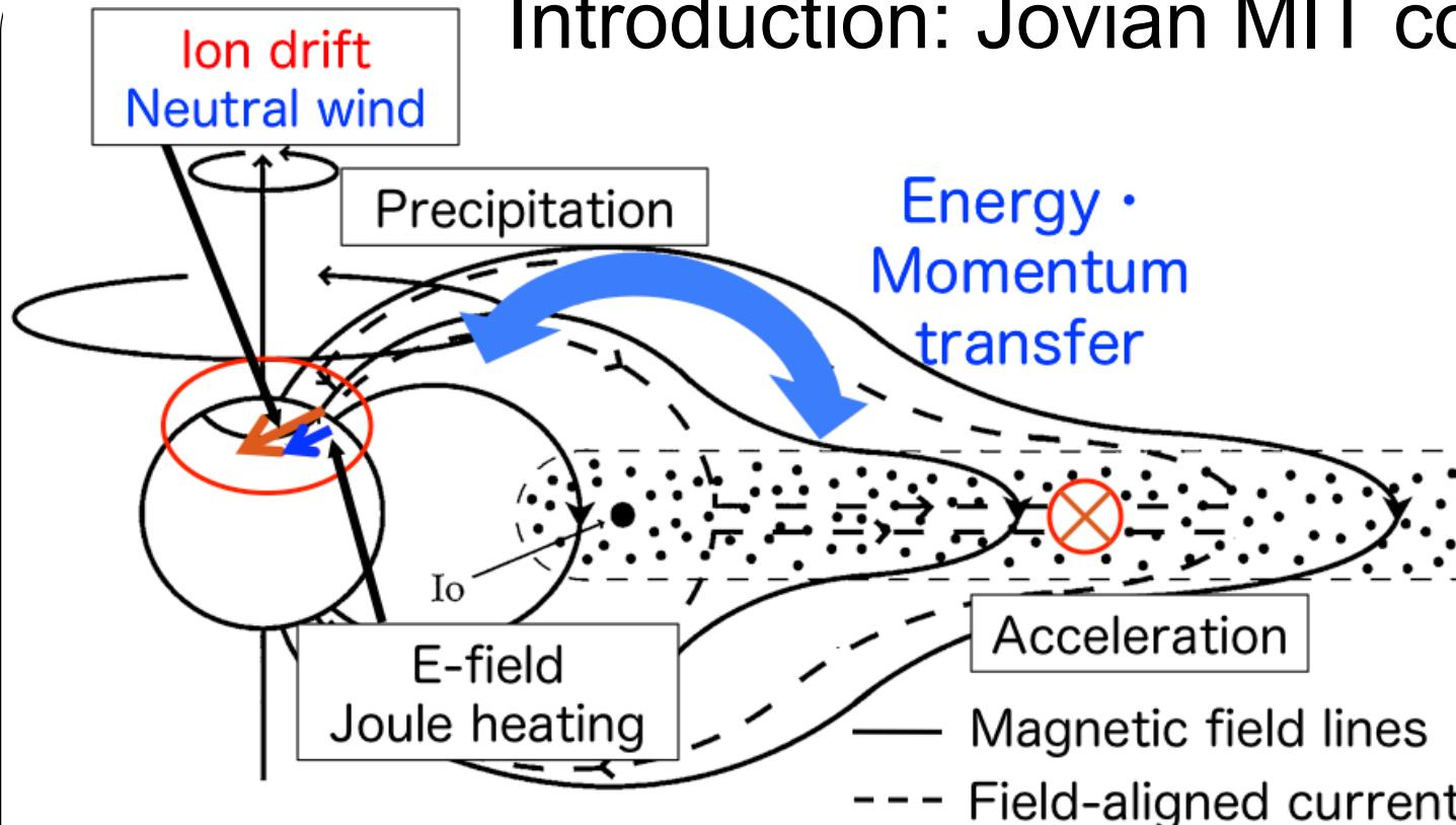
Fig. Mechanisms of the Jovian MIT coupling system (Cowley and Bunce, 2001)
