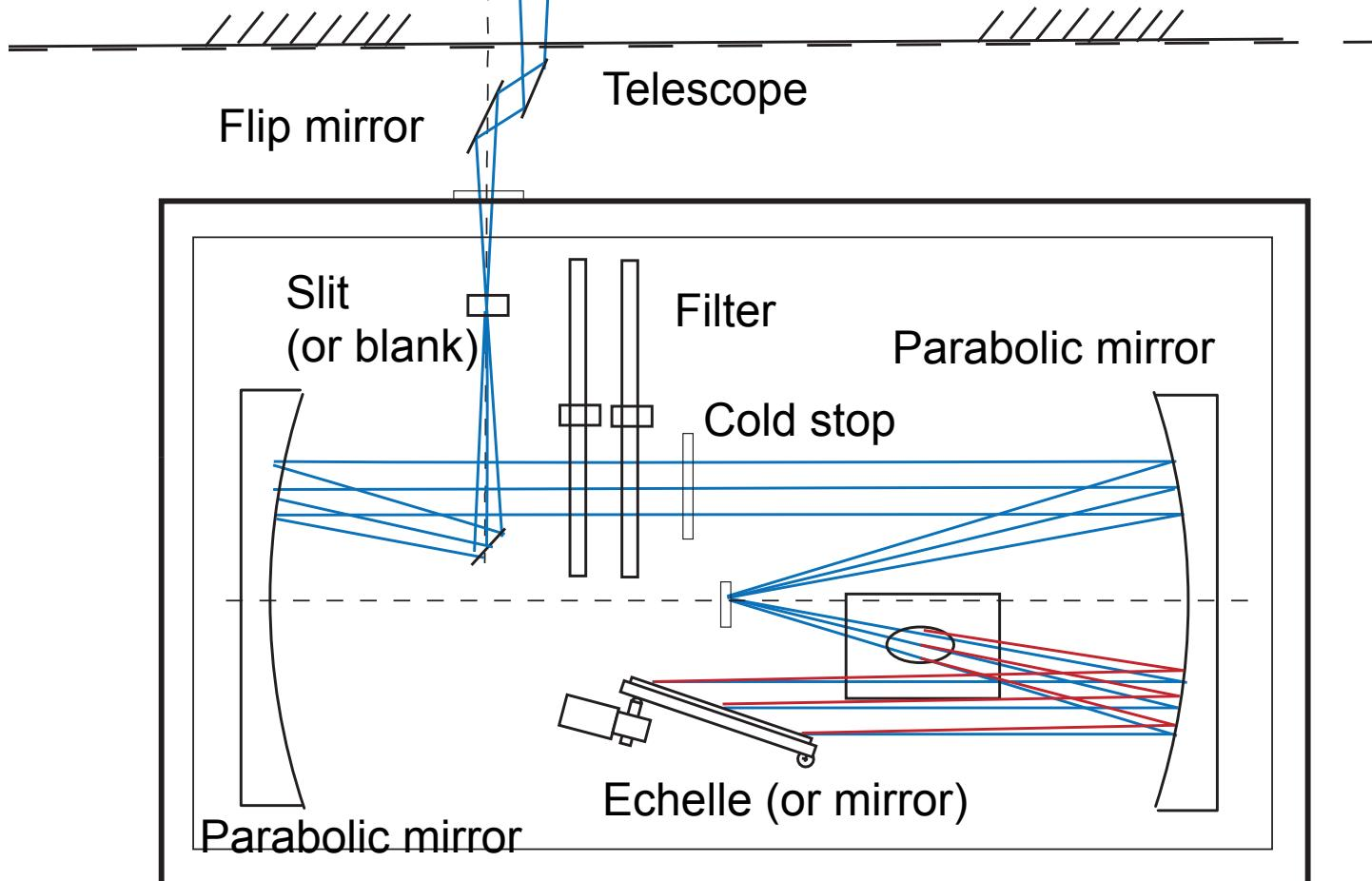
Fig. Optical Design of our spectrometer
